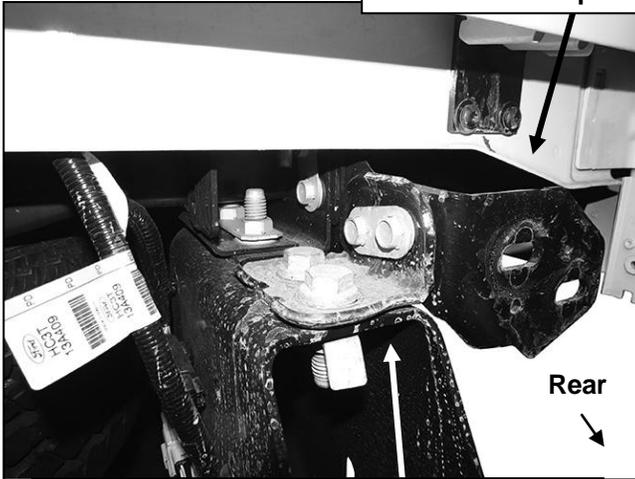
(Fig 4) Remove factory bumper brackets,
